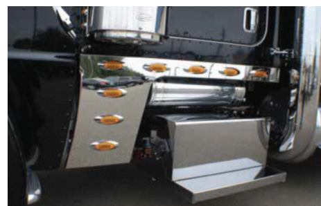
VP150104 PB - 379, 388, 389 BATTERY BOX - ALUMINUM
